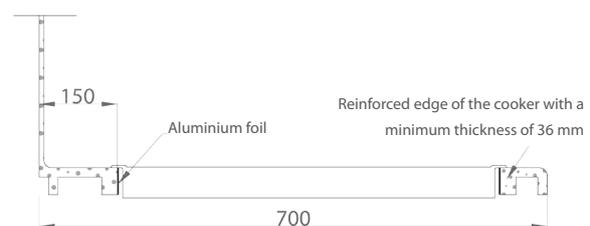
In case of a work counter that is 600 mm wide we can mount a wall cladding made of Kerrock material, but it should not be rigidly joined with a countertop. It is fixed elastically, as the picture shows.
