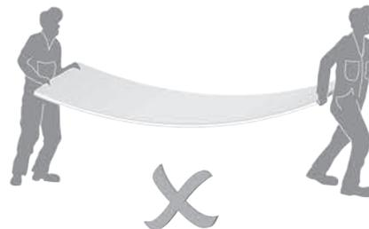
The sheets must be transported individually in a vertical position, where one hand serves as support and the other for control. It is recommended to use vacuum accessories for transporting heavy loads.
